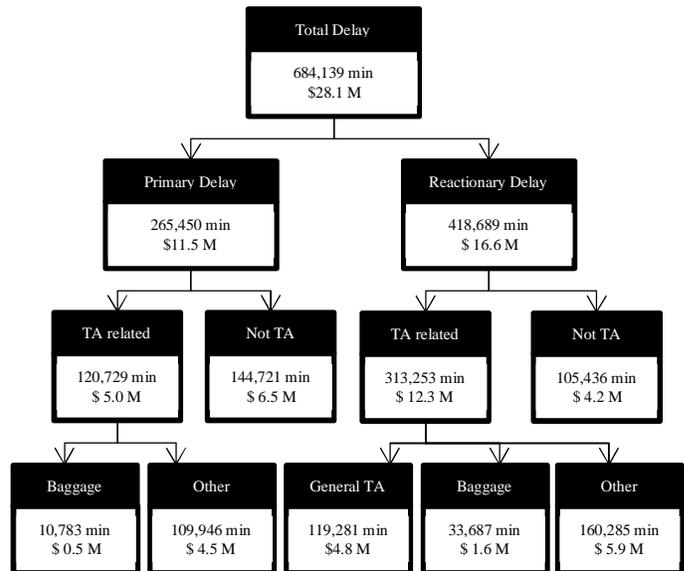
Fig. 4. Primary and reactionary delay cost breakdown while drilling down to aircraft Turnaround related and baggage related delays.
