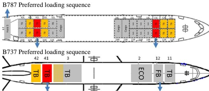
Fig. 13. Preferred Loading Sequence during pilot phase where HotCon and ShoCon baggage are given priority over terminating local baggage in order to be off-loaded first. (red TB: HotCon bags, MCT<50 min; orange TB: ShoCon bags, 50 min < MCT < 80 min, TB, Transfer bags MCT > 80 min; HUB Transfer bags for one dedicated flight; ECO terminating economy bags; FB, terminating business class and Sky Priority bags. Amended Figures Boeing [8],[9]
