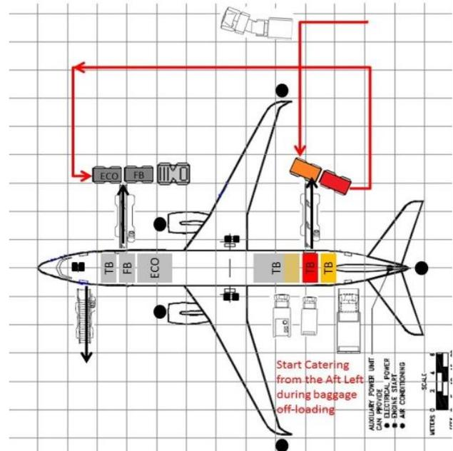
Fig. 15. B737 New off-loading process. Amended Figure Boeing [8]
