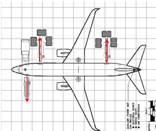
Fig. 14. Old situation B737 off-loading Amended Figure Boeing [8]
